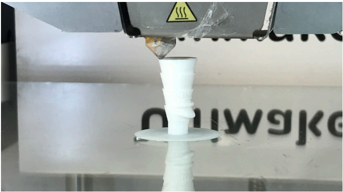
Figure 42: Material leaking during printing
