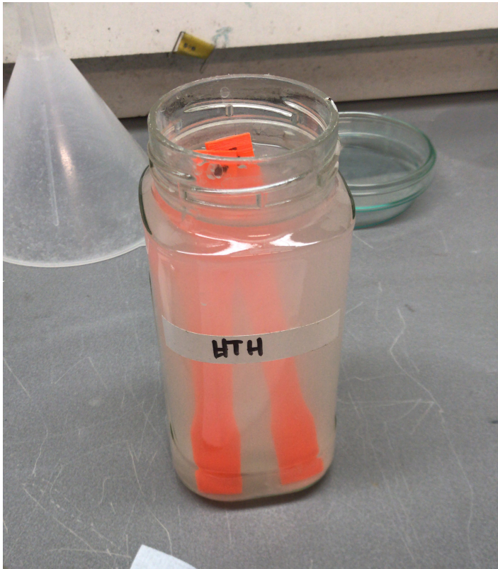
Figure 49: Samples soaked in a chlorine bath
