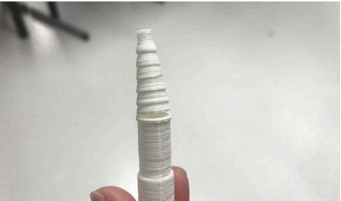
Figure 43: Fatal results of 100% fan speed
