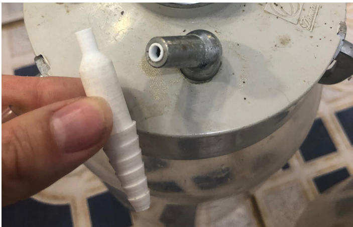
Figure 57: Broken connector at thinnest point
