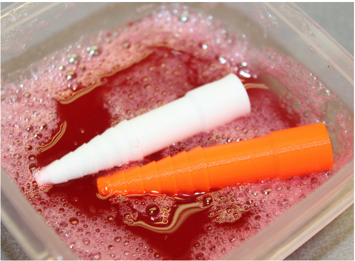
Figure 46: Connectors soaked in ATS
