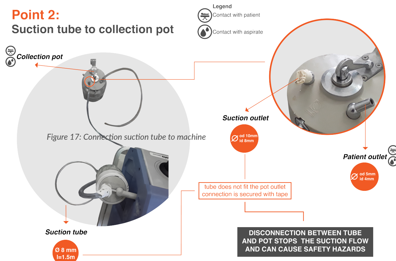
Figure 18: Connection suction tube to collection pot
