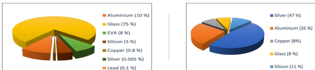
Figure 1.0 - Material distribution in c-Si solar panels according to weight ( left ) and economic value ( right ).
