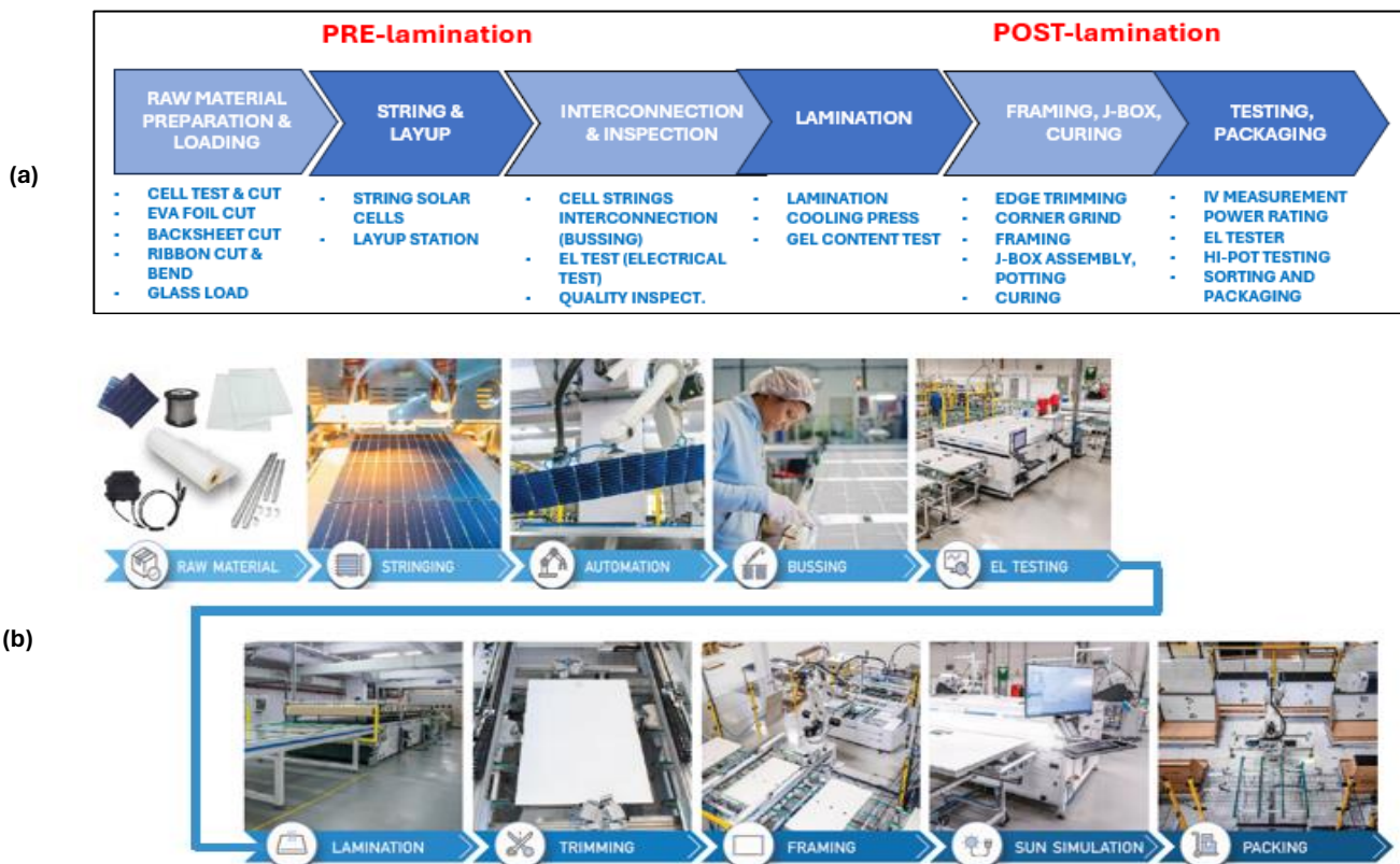
Figure 3.0 - Assembly process stream: (a) block sequence steps, (b) visuals of laminated PV module assembly flow (Adjusted from [16]).
