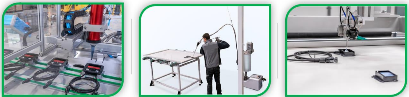
Figure 5.4 - Auto JB glueing (left), manual and auto JB potting (middle and right) [16]. Green contour: common to laminated lines.
