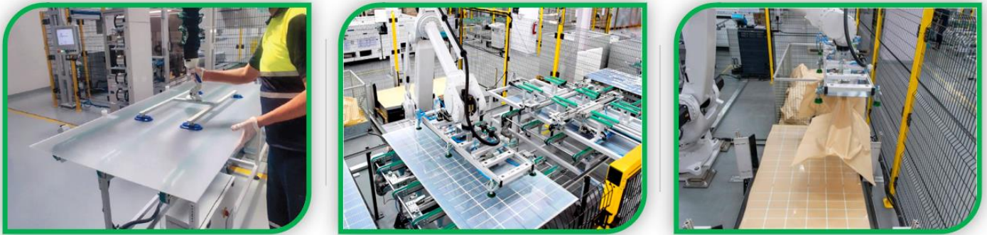
Figure 5.2 - Photographs of: Manipulator for glasses ( left ), automatic 2 nd glass layup robot ( middle and right ). (Source: Ecoprogetti – Catalogue, Sept. 2023 ). Green contours: common to standard and L-F module lines.
