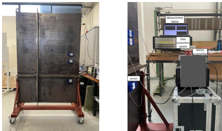
Fig. 4.: Experimental set-up. Instrumentation close-up (right).
