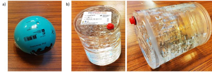
Figure 7: Phantoms used in the experiments. Note that the ball in a) is not completely spherical.
