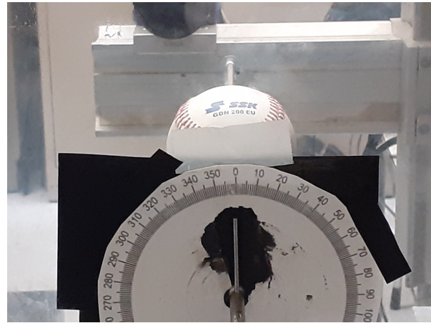
Figure 4.5: The angular control for the baseball
