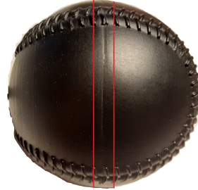
Figure 5.2: Photograph of the 3D printed baseball, where the dotted line indicates where the 2 halves are glued together. The smooth sphere has the same orientation, with the same vertical glue line vertical through the center of the baseball, when viewed from the side.
