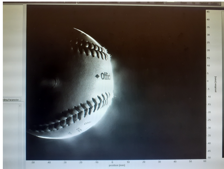
Figure 4.10: Field of view. The dimension is ca. 95mm by 115mm resulting in a magnification factor of 0.15
