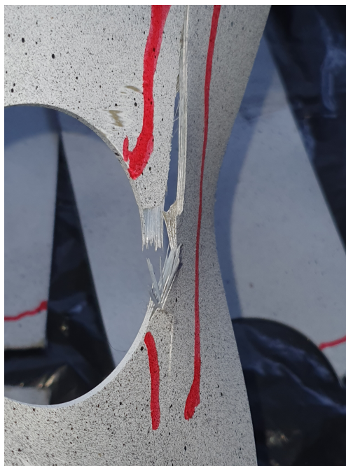
Figure 5.16: Longitudinal crack in de applied load direction. Failure surface and delamination in sample D60.
