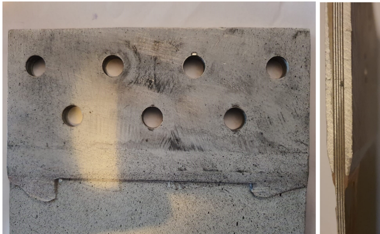
Figure 4.1: Aluminum tabs on the specimens.
