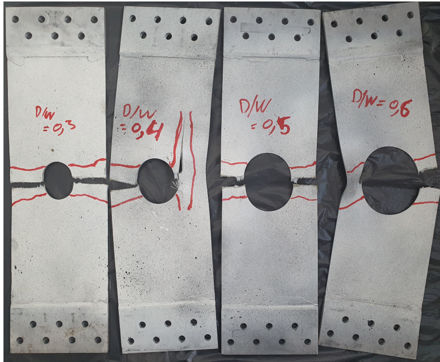
Figure 5.12: The four glare samples used and their delamination boundaries.
