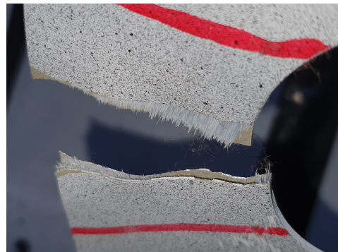
Figure 5.14: Failure surface of sample D75.
