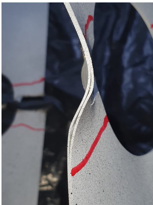
Figure 5.15: Delamination in sample D90.
