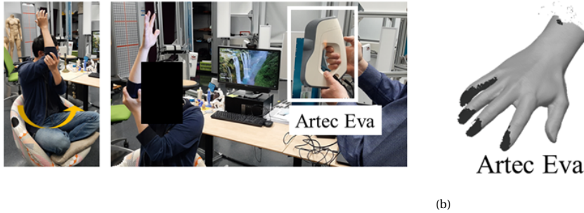
Figure 8.2: 3D scanning of human hands using Artec® Eva® scanner, courtesy of [312].
