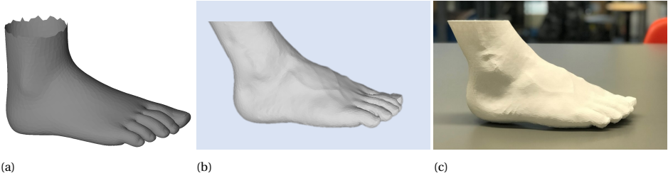
Figure 5.7: No-load foot. (a) The source mesh. (b) Scanned through Artec Eva scanner. (c) Printed Artec Eva output via Ultimaker S5 printer.
