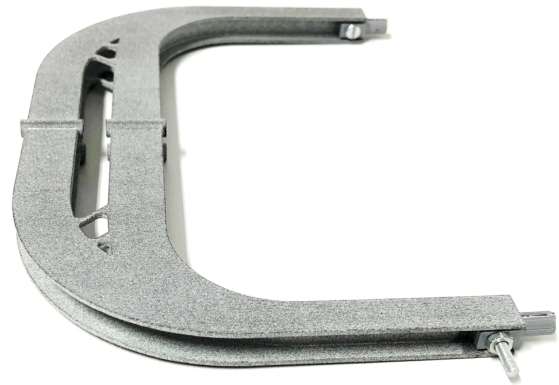
Fig. 8. Side view of the prototype fabricated using Multi Jet Fusion from Polyamide 12
