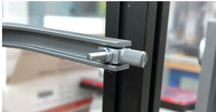
Figure A.7: 3D printed connection between mechanism and Cardan.
