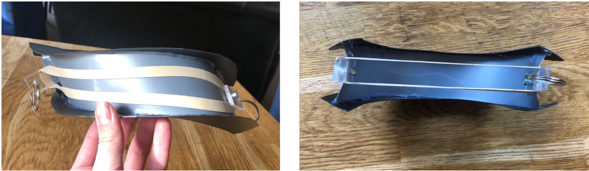
Figure B.4: Prototypes using elastics to create pre-stress in the structure
