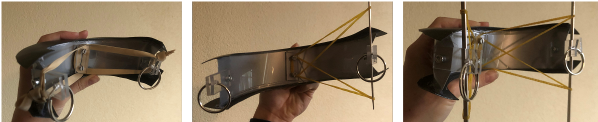
Figure B.5: Prototypes using elastics to create pre stress in the structure
