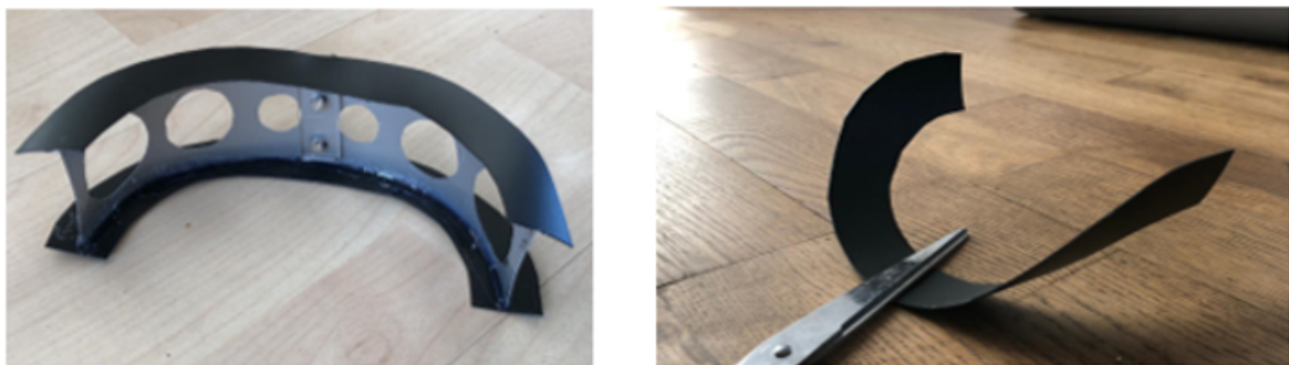
Figure B.3: Prototypes using pre-curved flanges to obtain pre-stress in the structure
