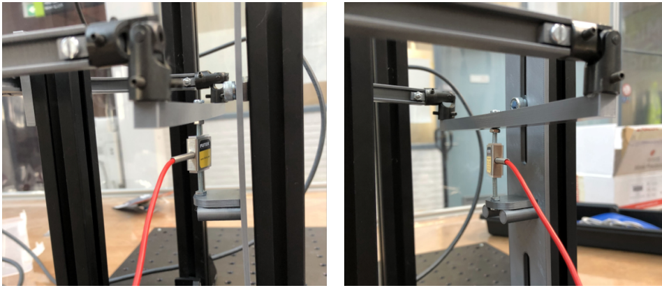
Figure A.8: Experimental setup for bending with 3D printed beam
