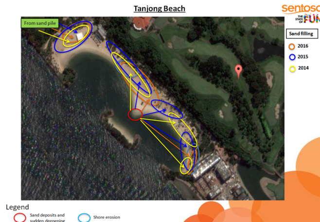
Figure 16: The performed maintenance by the Sentosa Development Corporation. Sediment from the tombolo has been distributed over the (mostly) exposed coastline and sediment has been added from the stockpiles. (Sentosa Development Corporation, 2016)
