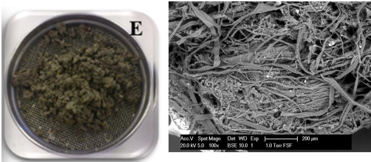
Figure 2.2: (Left) A picture of raw FSF (Ghasimi et al., 2016). (Right) Scanning electron microscopic picture of raw FSF from WWTP Blaricum (Ghasimi et al., 2015).
