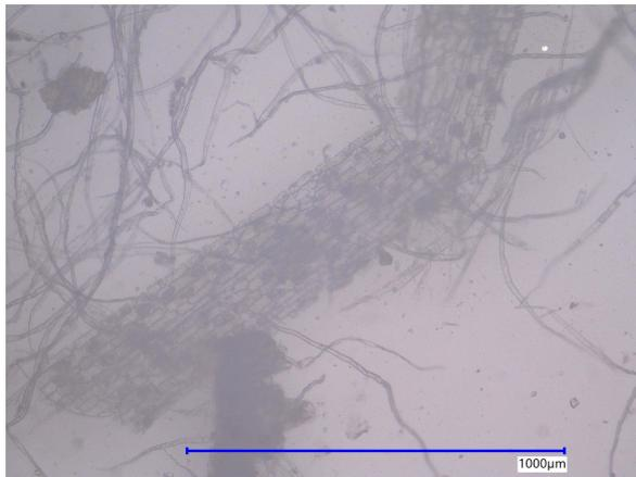
(a) fibers, sludge flocs and plant cells found in the fFSF sample.
