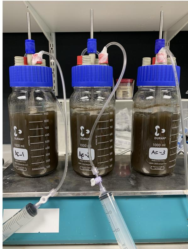
Figure 3.6: The experiment set up for batch activity test. The tests were performed in duplicate. Each Duran® bottle was equipped with a gas inlet, gas outlet, sampling port and electrode probe port (for pH and DO measurement).
