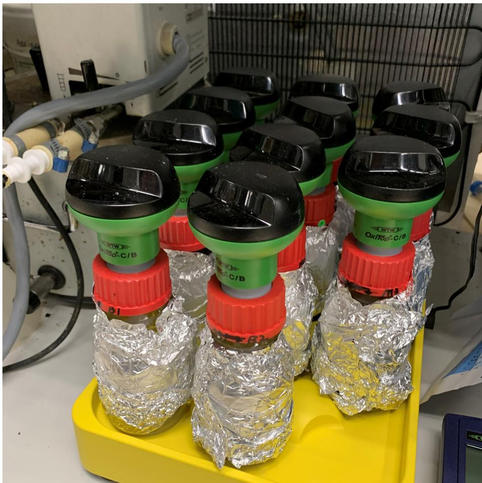
Figure 3.4: Oxitop® system for BOD measurement. Aerobic biodegradation was taken place in 250 mL Duran® bottles. These bottles were connected to Oxitop® pressure measuring heads and covered with aluminium foil to prevent the growth of algae.
