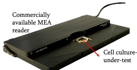
Figure 7.3: Commercially available MultiChannel Systems MEA recording setup. [8].
