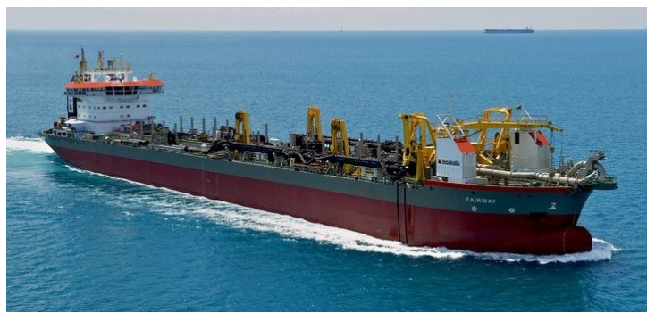
Figure E.4: Trailing Suction Hopper Dredge 'Fairway'.
