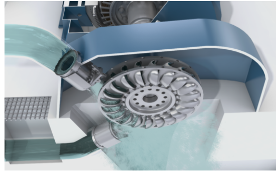
Figure I.2: Hydro impulse turbine (Pelton) designed for high head differences (between 200 m and 1800 m). Power output could be up to 350 MW. Source: GE Renewable Energy.
