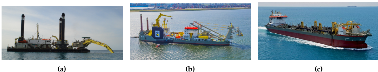
Figure D.1: Type of equipment related to dredging activities: (a). Back Hoe Dredger (BHD), (b). Cutter Suction Dredge and (c). Trailing Suction Hopper Dredge (TSHD).
