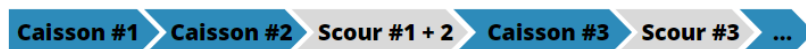
Figure G.2: Schematic planning of the construction sequences taking into account the difference in workability and wave conditions.
