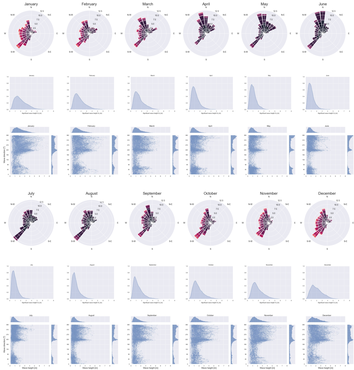
Figure A.11: Seasonal variability in wave conditions for the desired location, shown in three types of monthly graphs: a windrose, a probability density function for the wave height and a wave direction versus wave height distribution.
