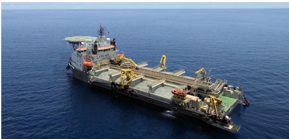
Figure E.14: Dynamic Positioned (DP) Side Stone Dumping Vessel the Ndeavor.
