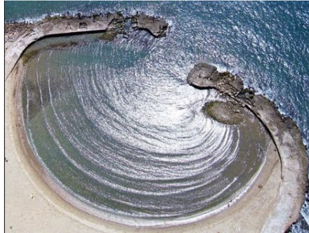
Figure 7.1: Diffraction phenomenon of ocean waves encountering a break water, after which waves are spread out and changing direction in the basin.
