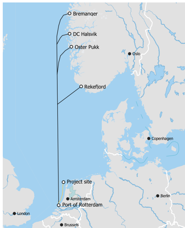
Figure E.8: Chart of the transportation of rock material from quarries in Norway to the Port of Rotterdam in the Netherlands by bulk carrier (in black), afterwards it is loaded onto the FPV and transported to project site (in orange).
