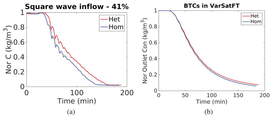
Figure 4: Normalized concentration against time duration for square wave intermittent infiltration in 41% of maximum pump flow rate on lab scale (a). VarSatFT validation for lab results (b).
