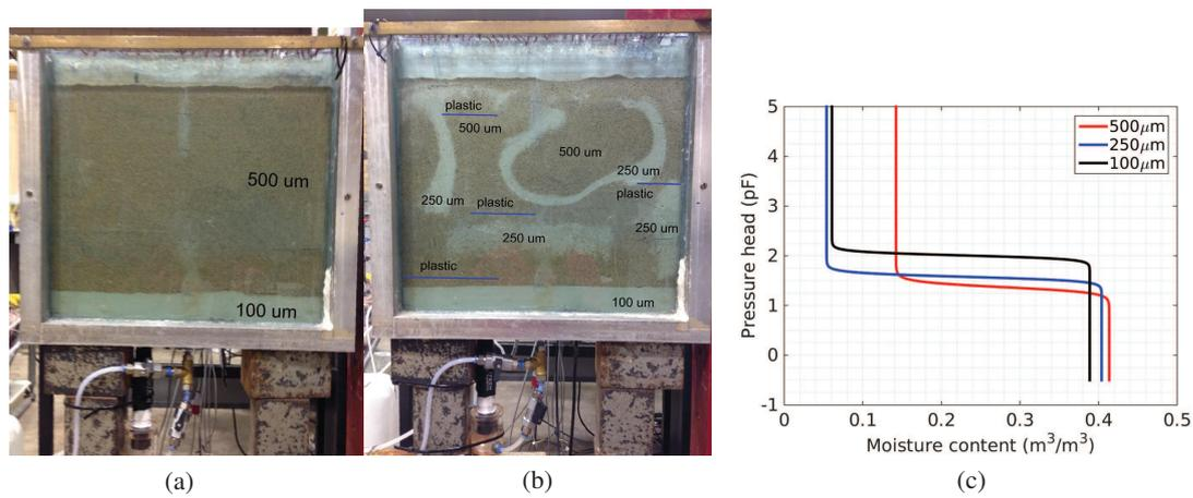
Figure 2: Laboratory scenarios for Homogeneous (a) and Heterogeneous (b) domains. Water retention curves optimized using DREAM<sub>ZS</sub> for sands of size 100 μm, 250 μm and 500 μm (c).
