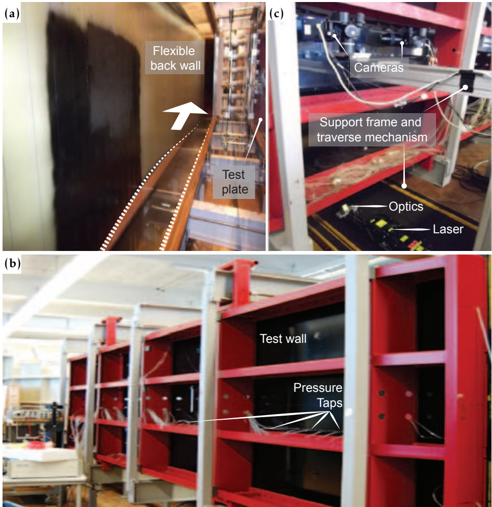
Figure 4.7: (a) Internal test section view displaying the curved back wall with blackened section and illustrating the general flow direction; (b) external view of the test section and (c) PIV setup.
