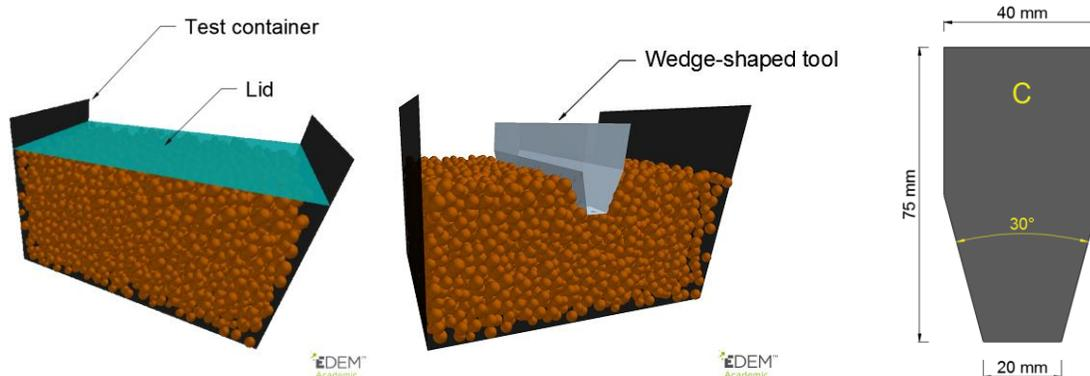
Figure 1. Virtual apparatus in EDEM2018. Left: the consolidation stage; middle: the penetration stage; right: wedge-shaped tool
