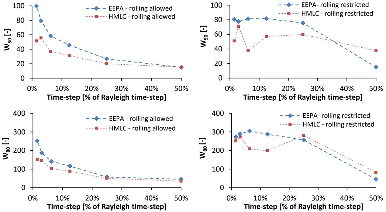
**Figure 2. Influence of time-step on the dimensionless penetration resistance. Left: rolling is allowed; right: rolling is restricted**
