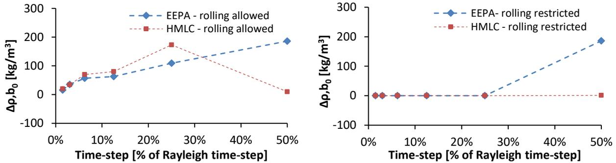
Figure 3. Influence of time-step on the bulk density change in the loose condition. Left: rolling is allowed; right: rolling is restricted
