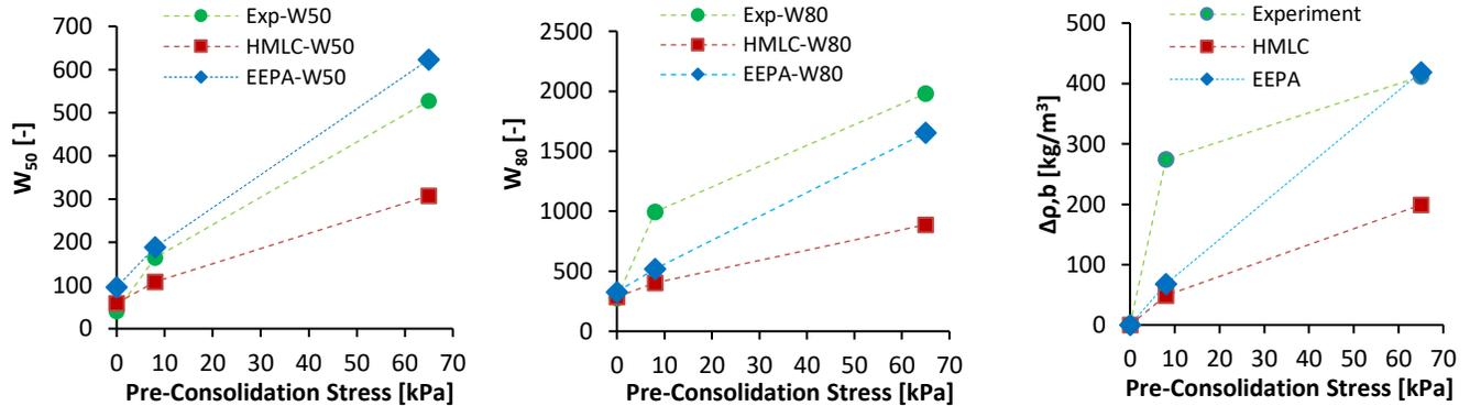
Figure 4. Effect of pre-consolidation stress on the penetration resistance. Left: Dimensionless penetration resistance at depth of 50 mm; right: Dimensionless penetration resistance at depth of 80 mm
