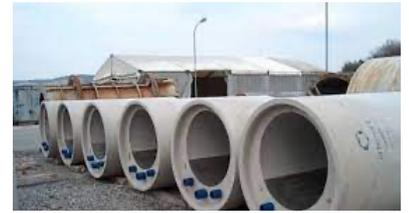
Figure 8 - Riothermal energy recovery from sewerage
