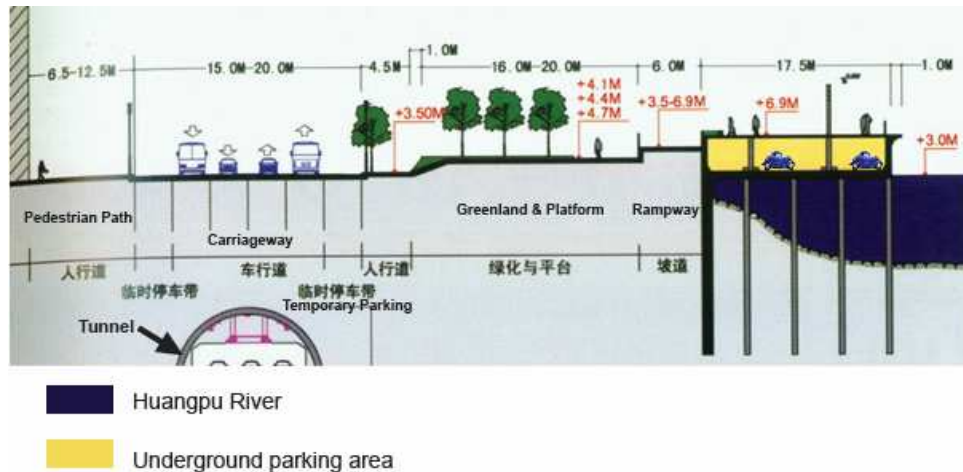
Fig.2. 19 Cross section of waterfront area in Bund of Shanghai (Xi and Xu, 2011)
