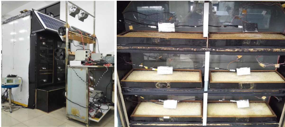
Figure 4.9: Testing rig of the SPDW (Left). The desiccant beds are integrated within the window (Right).
