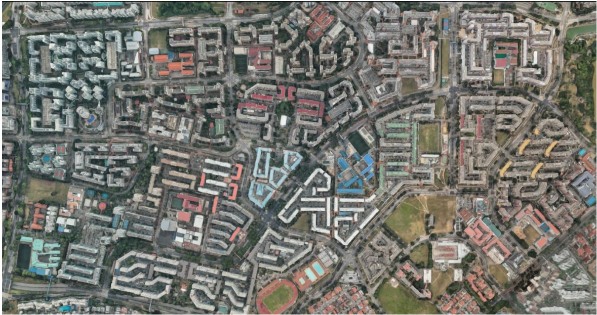
Figure 2.17: Bird's eye view of slab blocks aligning with the sun path. (Source: Google Maps)
