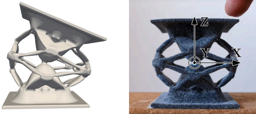
Fig. 1. Computational design of a multi-axis flexure and its prototyped counterpart. The flexure is compliant in the rotations about the x and y -axis while stiff in the x , y and z translations as well as rotation about the z -axis.
