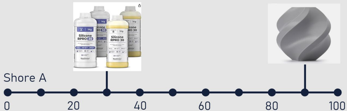
Figure 41 Shore A value scale with the tested materials shown.
