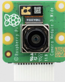
Figure 39 The Pi Camera 3 Wide is used in the robot
