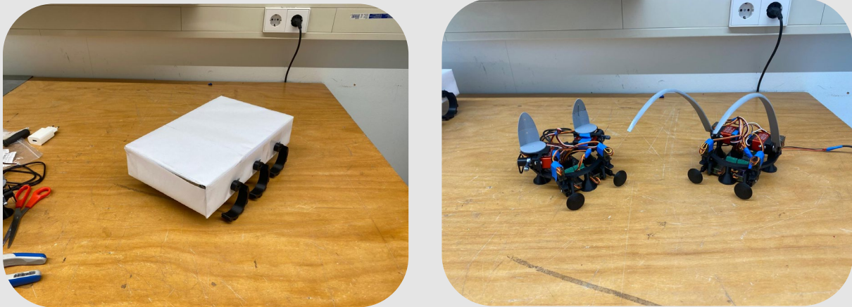
Figure 25 Mockup of the LZ robot (left), modules of ears and eyes on the left, and antennae and eyes on the right (right).
