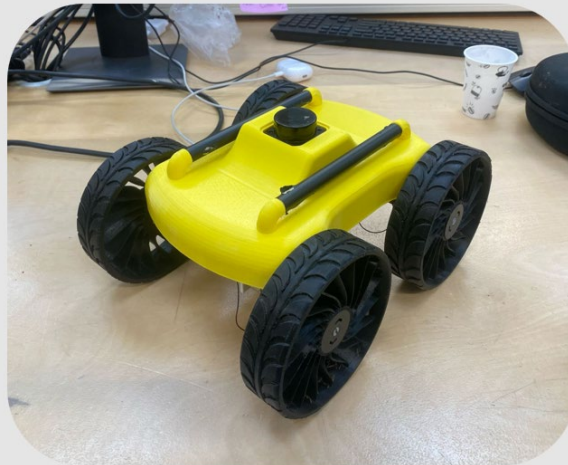
Figure 44 Picture of the robot frame used for the locomotion of this project
