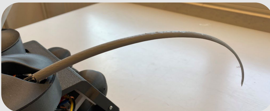
Figure 42 Picture of the prototype antenna used in the robot
