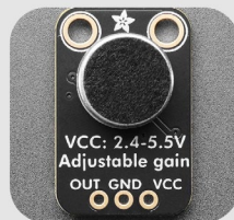
Figure 40 The Adafruit MAX4466 microphone used for the robot
