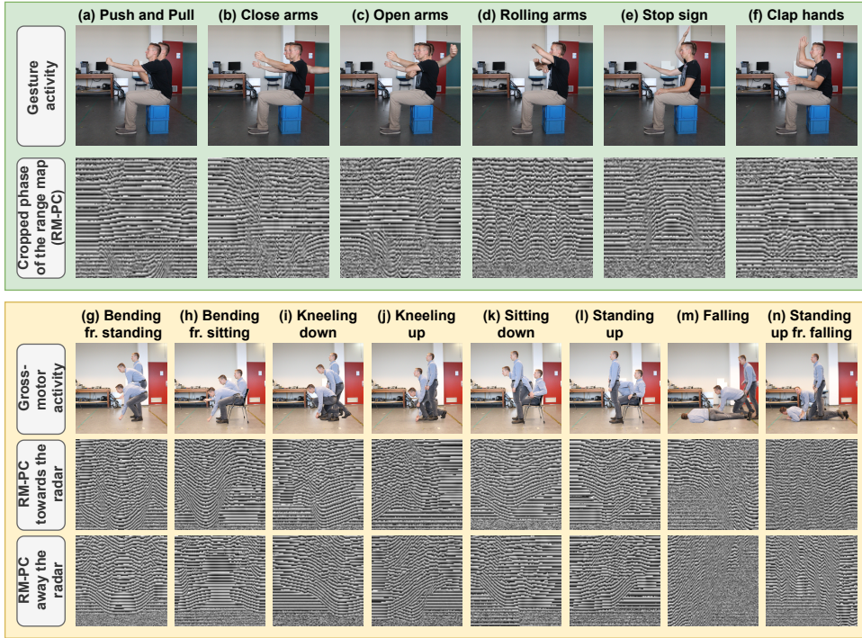
Figure 3.6: Pictures of the activities and related cropped phase matrices: six gestures (top, green-shaded), and eight gross-motor activities performed bidirectionally (bottom, yellow-shaded).
