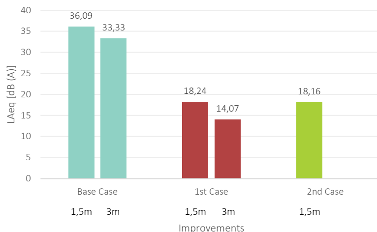
Figure 97. A-weighted Sound Pressure Level performance per distance per case.
