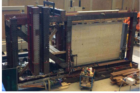
Figure 3: Setup for in-plane tests on timber diaphragms
