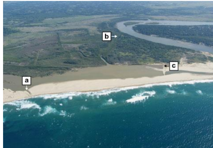
Figure 2.3: Photo of the Mfolozi River and St Lucia mouth region showing main management interventions: (a) weak link at Mfolozi Mouth and Indian Ocean, (b) back channel and (c) construction wall (Whitfield & Taylor, 2009)
