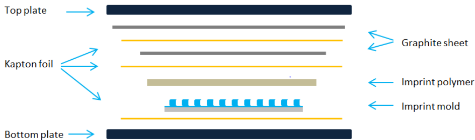
Figure A.5: Overview of the layer buildup for imprinting large samples.
