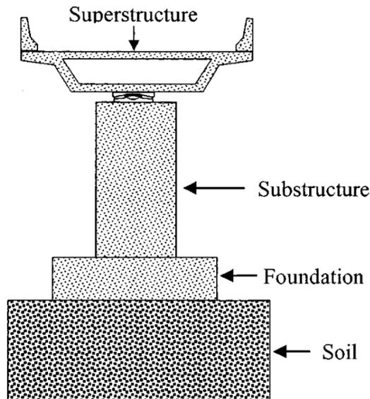
Figure 2.6: Components of a bridge [Dicleli et al., 2005]
