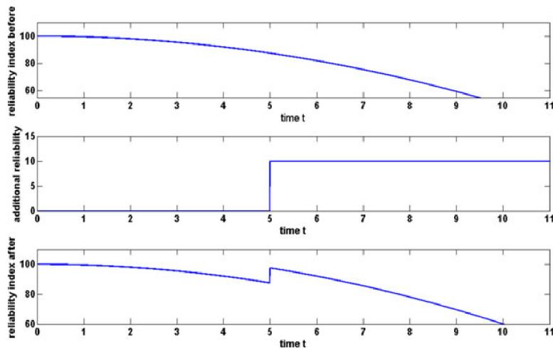
Figure 2.3: Reliability index before (upper) and after (lower) maintenance, including the additional reliability profile due to maintenance (middle) [Ng et al., 2009]
