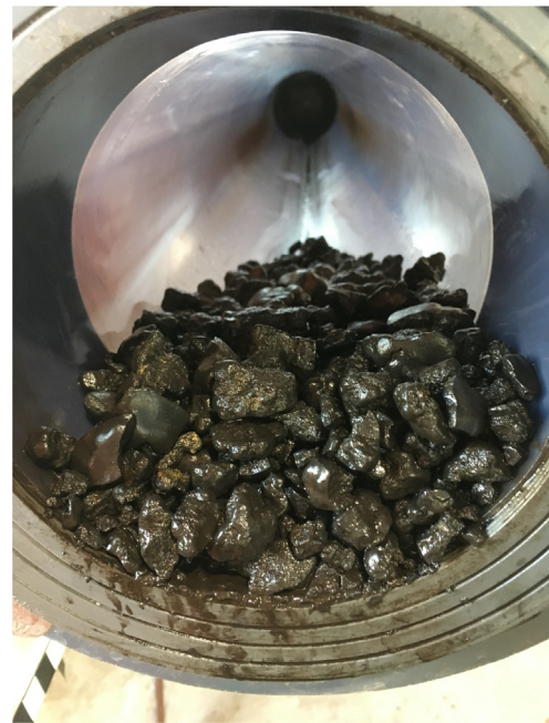
Fig. 6. A bed of nodules placed in the tilting pipe setup.
