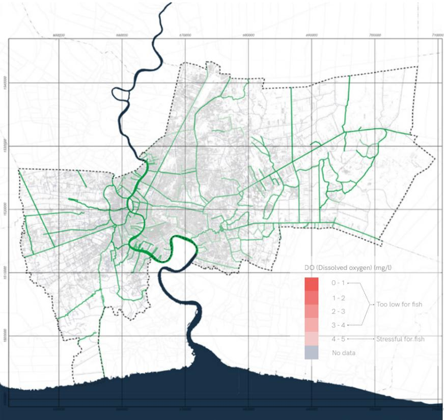
If BOD is high, it means that microorganisms are using most of the oxygen, resulting in difficulties for larger aquatic animals to survive (Ipsaro, n.d.). Whereas DO is the amount of oxygen in the water, it is a significant measure of water quality since it is a direct index of an aquatic resource's ability to support life (US EPA, 2013). Therefore, the lower DO is, the more inferior the quality of water is.
