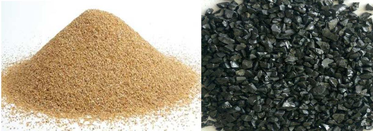
Figure 23. Sand (left) and anthracite (right) as filtration medium (IndiaMart, 2018)
