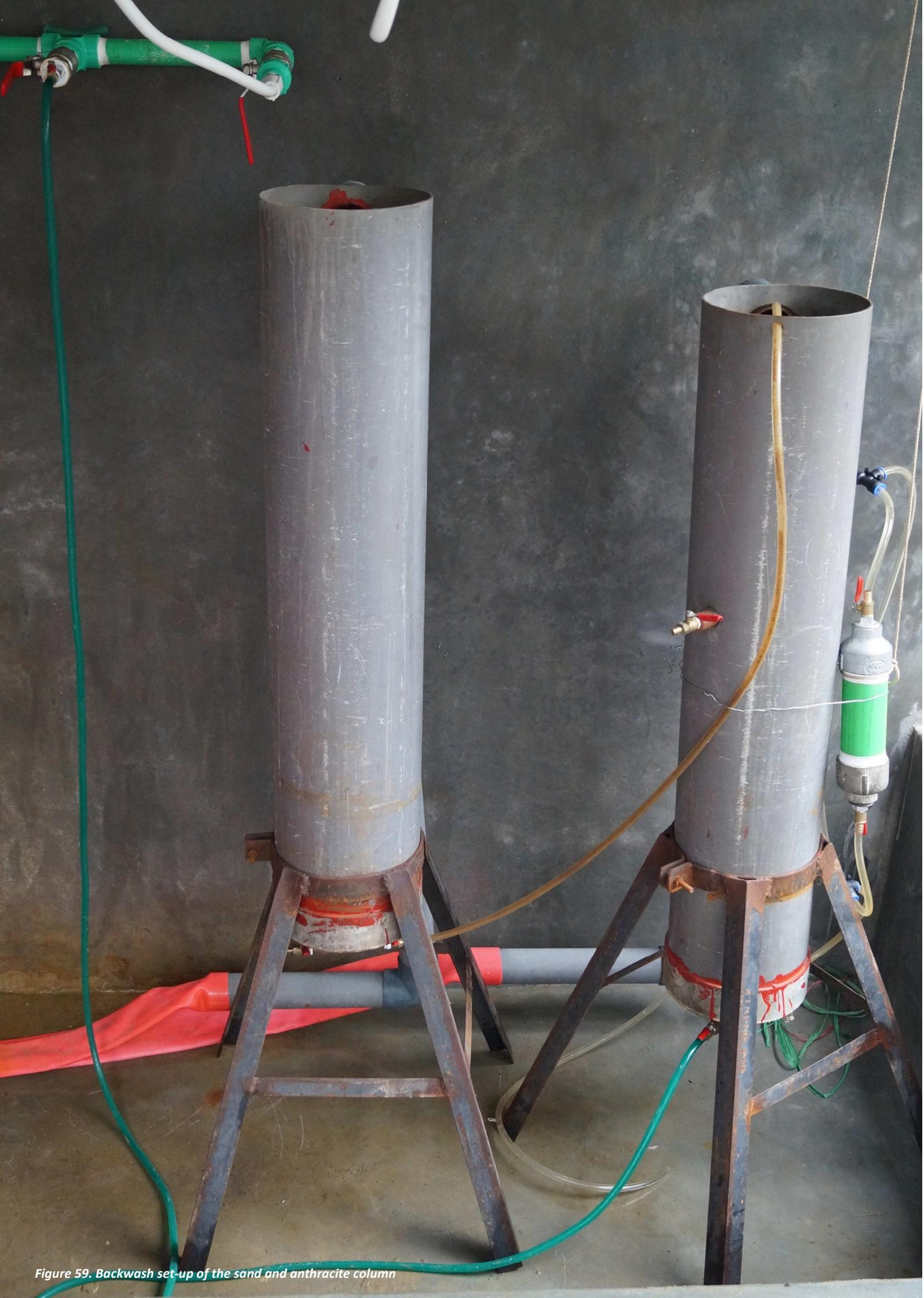
Figure 59. Backwash set-up of the sand and anthracite column
