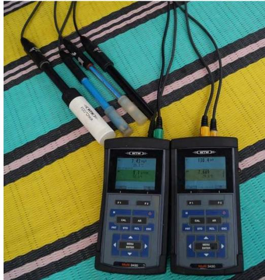
Figure 26. WTW Multi3430 multimeter
