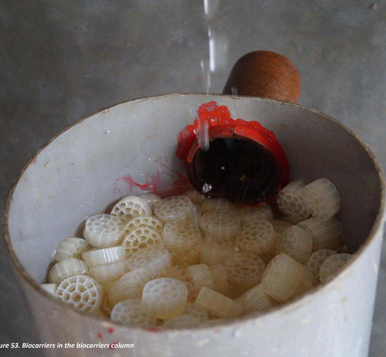
*Figure 53. Biocarriers in the biocarriers column*
