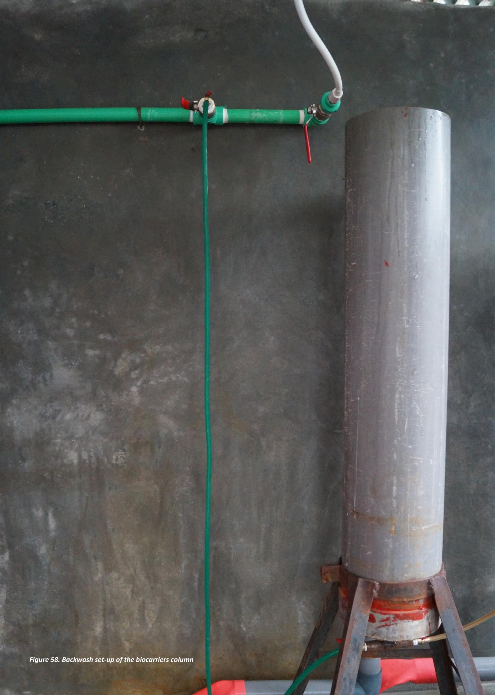
Figure 58. Backwash set-up of the biocarriers column
