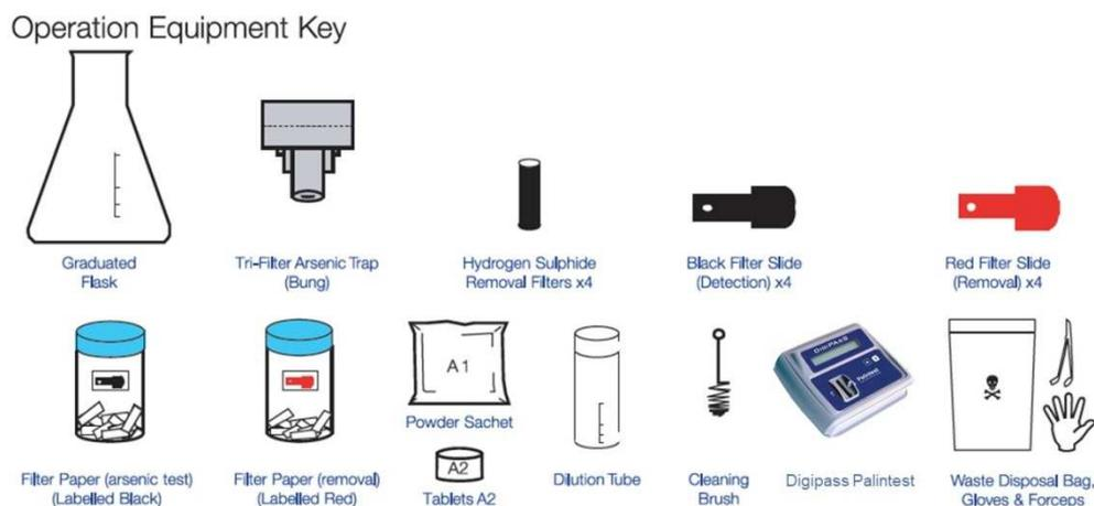
Figure 24. Operation equipment of the arsenator
