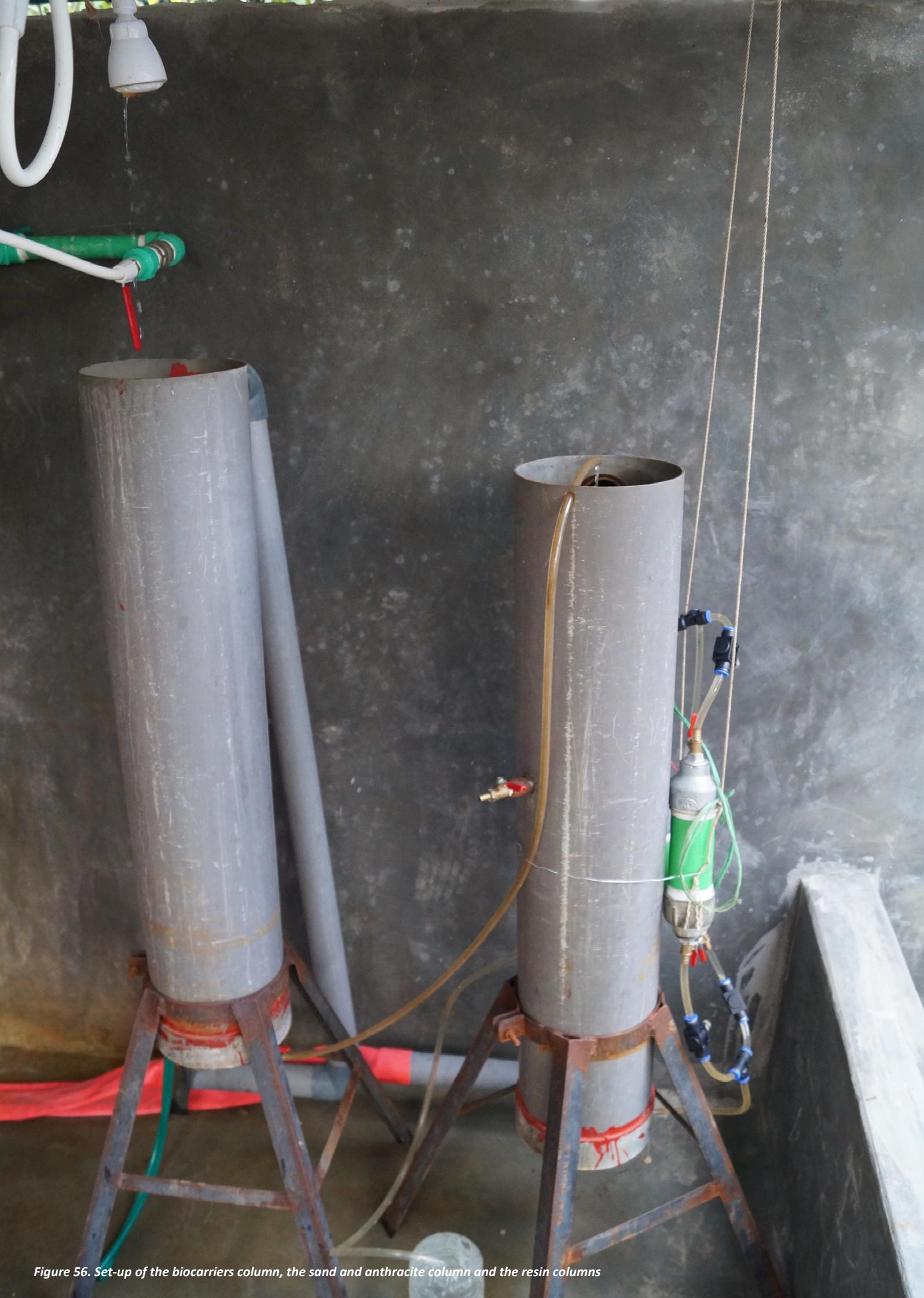
Figure 56. Set-up of the biocarriers column, the sand and anthracite column and the resin columns
