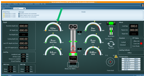
Fig. 6. The dashboard as seen by the drillers during production. To indicate the values predicted by the algorithm indicators have been added above the gauges as shows with the arrow.
