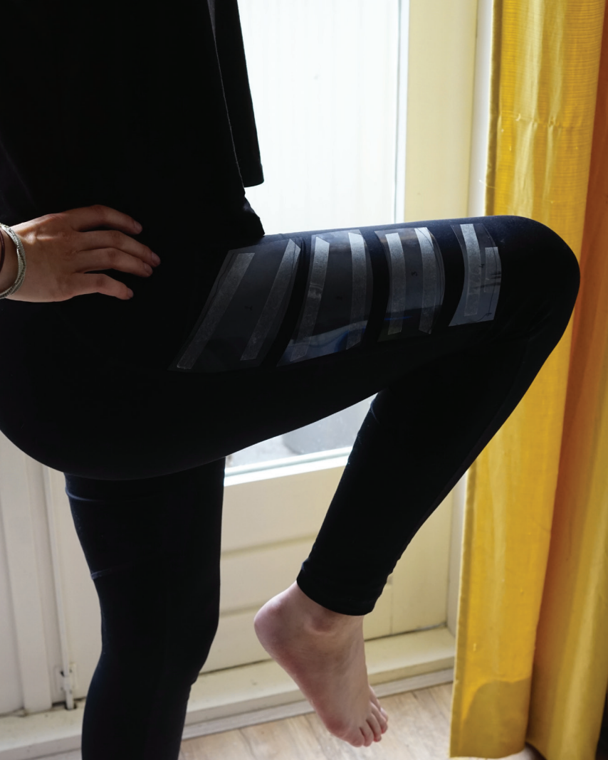
figure 93: Plastic sheets on a legging to test the stretch and comfort
