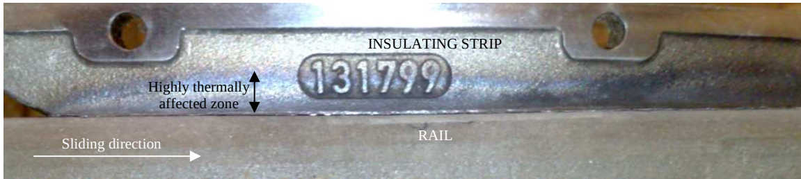
Fig. 4B.21. Photograph of an insulating strip after testing and cleaning.
