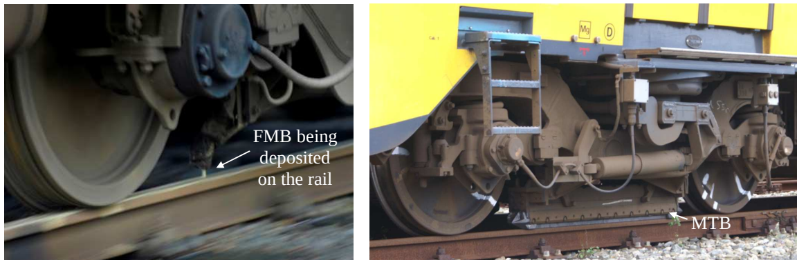
Fig. 1.9. Photograph of: (a) trainborne application of FMB in the Netherlands [1.44]; (b) MTB in active position of the VIRM train of NS.
