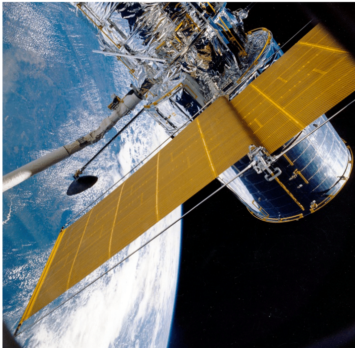
(a) The ESA/B Ae flexible solar array utilized on the Hubble Space Telescope, relying on central bi-stem masts for tensioning [23]
