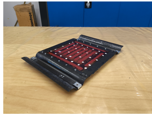
(b) Rear view showing adhesive lines
