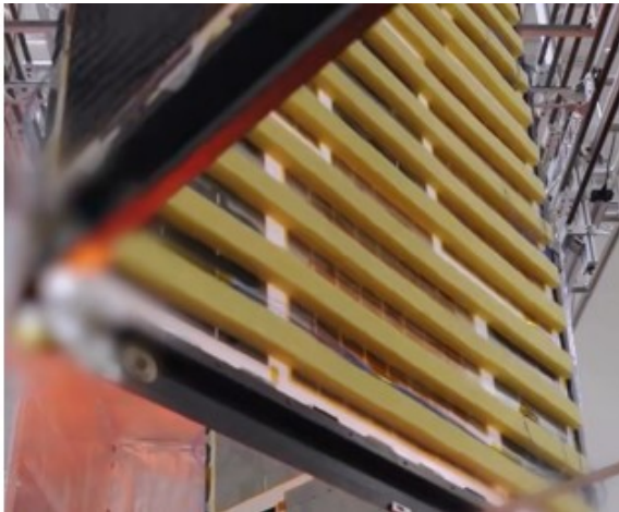
(a) Unfolding ELSA array showcasing polyimide foam strips [68]
