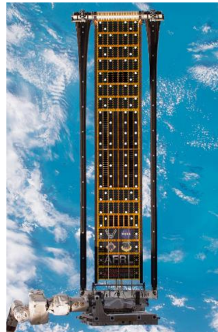
(b) The modern Roll-Out Solar Array (ROSA), utilizing perimeter tensioning via composite slit-tube edge booms [17]
