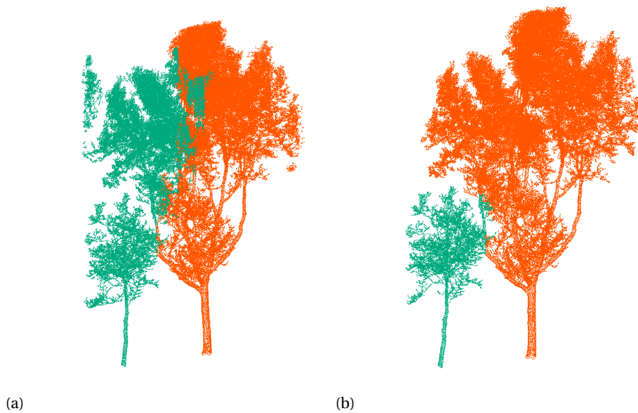
Figure 5.17: Tree separation details of the existing method and the proposed VoxTree method from TLS point cloud. (a) Separation results of Wu's method. (b) Separation results of the proposed VoxTree method.
