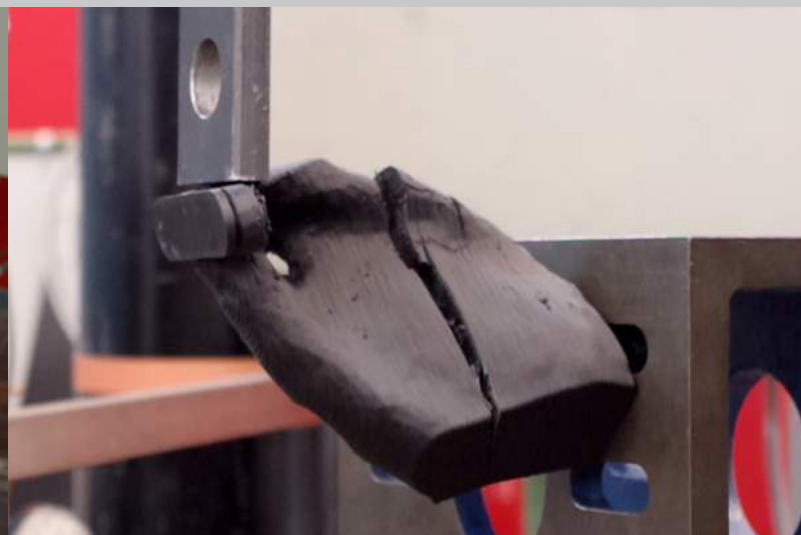
Figure 6.12 - Failed part loaded in Y-direction
