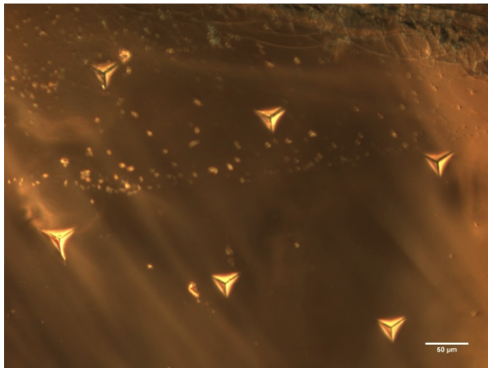
Figure E.8: Sample 40\text{KPO}_3\text{-}20\text{B}_2\text{O}_3\text{-}25\text{FA-}15\text{Al}_2\text{O}_3 under 2.N.
