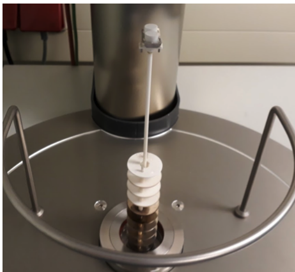
Figure A.3: Sample carrier with two alumina pans: one for the measured glass and another to be used as a reference.
