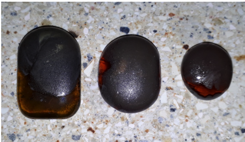
Figure 4.24: Pure slag melted at 1500\text{ }^\circ\text{C} using the melt-quenching technique.
