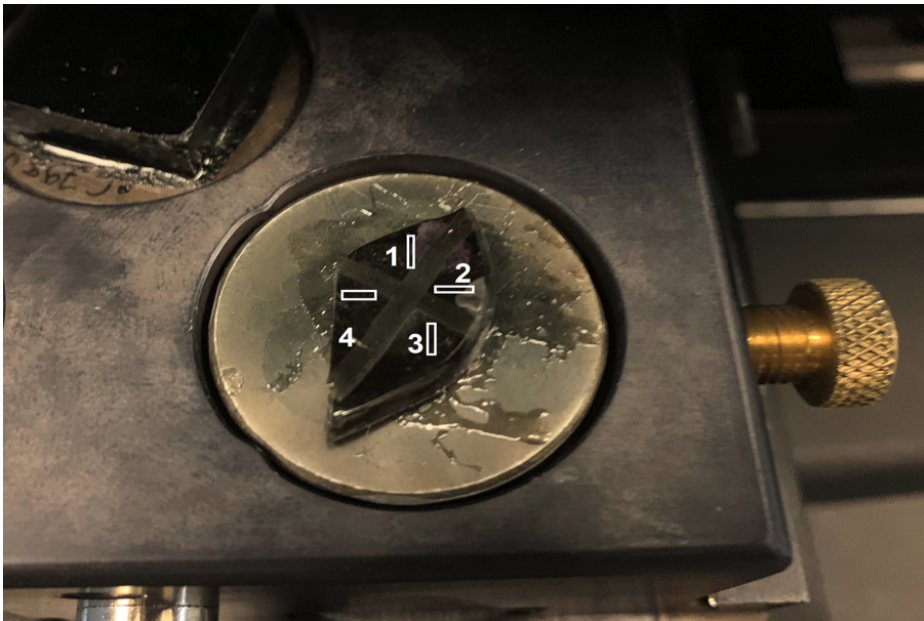
Figure 6.20: Sample 40\text{KPO}_3\text{-}20\text{B}_2\text{O}_3\text{-}25\text{fly ash-}15\text{Al}_2\text{O}_3 divided in four areas tested in different directions in the indentation test.
