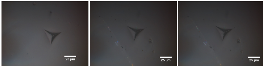
Figure E.30: Three indents of the sample 50KPO 3 -20B 2 O 3 -15Slag-15Al 2 O 3 under 2N, analysed by reflected light.
