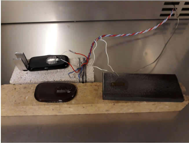
Figure 5.6: Setup of test 5, steel (channel 1), 75\text{KPO}_3\text{-}12.5\text{Slag-}12.5\text{Al}_2\text{O}_3 (channel 2) and 60\text{KPO}_3\text{-}20\text{Slag-}20\text{Al}_2\text{O}_3 (channel 3).
