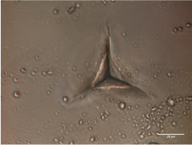
Figure 6.12: Indent of the sample 75\text{KPO}_3\text{-}12.5\text{slag-}12.5\text{Al}_2\text{O}_3 .
