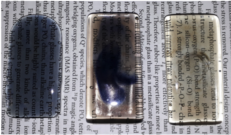
Figure 4.9: Samples consisting of 12.5% slag melted at different temperatures: 1150 °C, 1250 °C, and 1350 °C, respectively.
