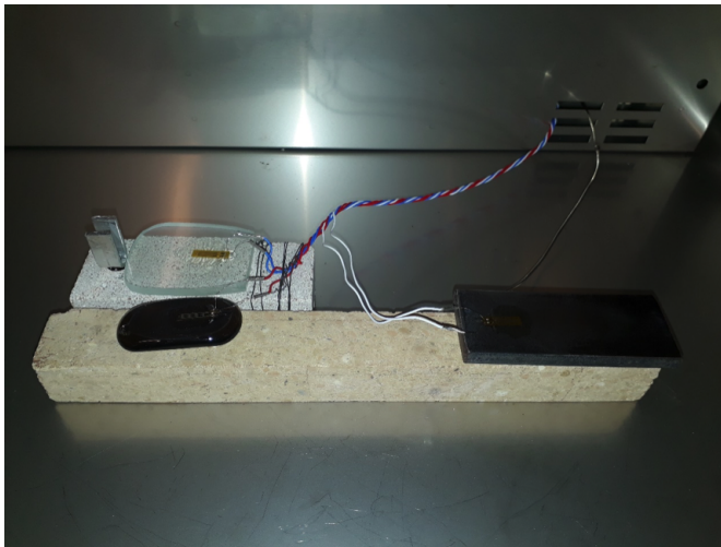
Figure 5.7: Setup of test 7, steel (channel 1), 50\text{KPO}_3\text{-}10\text{B}_2\text{O}_3\text{-}25\text{FA-}15\text{Al}_2\text{O}_3 (channel 2) and soda-lime (channel 3).
