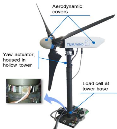
Figure 3. The G1 wind turbine with highlighted components.
