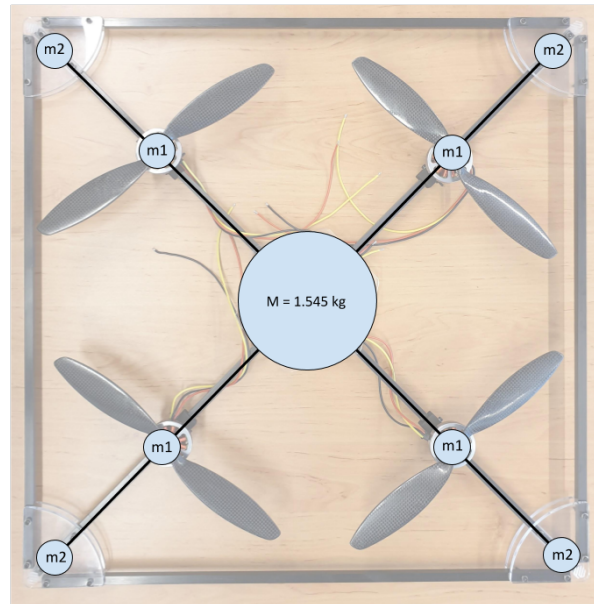
Figure 5.4: Inertia model with cylindrical mass M in the centre and point masses m1 and m2 as motor assembly and corner assembly
