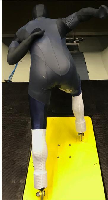
Figure B.1: Figure of the skating suit used for the PIV and IT measurements.
