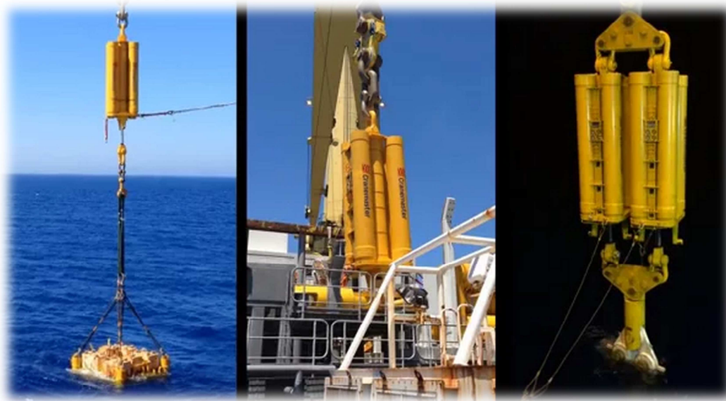
Figure 5-1 - "Cranemaster Passive Heave Compensator"
