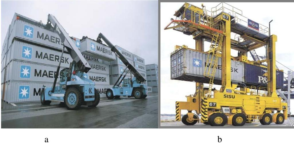
**Figure 3-6 Pictures of RS (a) and SC (b) (Source: APMT)**
