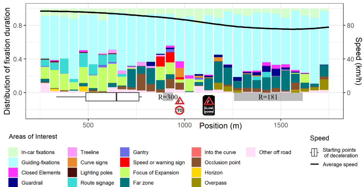
Figure 5-14 Average speed behaviour, distribution of fixation duration, and start of deceleration distribution of Curve 5, having a horizontal radius of 300 m. The positions of the curve is indicated with a grey box and the positions of speed and warning signs are also indicated.
