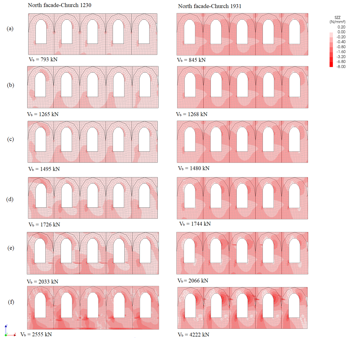
Figure 9.15: Compressive stresses for the due to pushover loading for the Northern facades, [scale factor=0.05]
