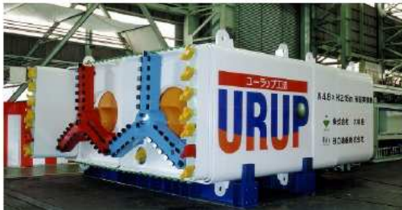
Figure 5; The TBM used at the pilot project
