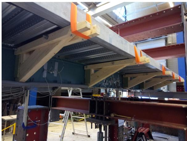
Figure 4.17: Wooden cantilever supporting structure
