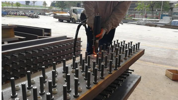
Figure 2.1: Welding of a stud connector using a welding gun
