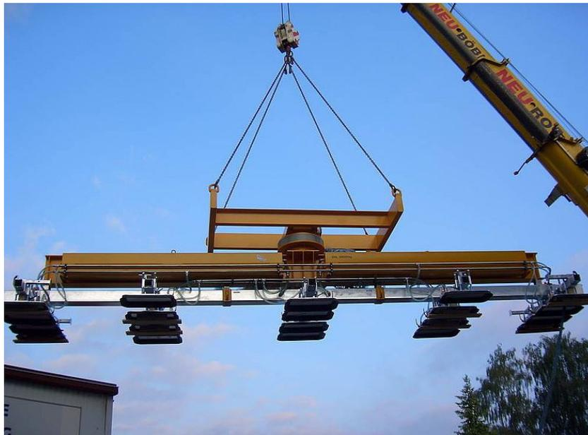
Figure 4.43: Vacuum lifter - up to 20000kg
