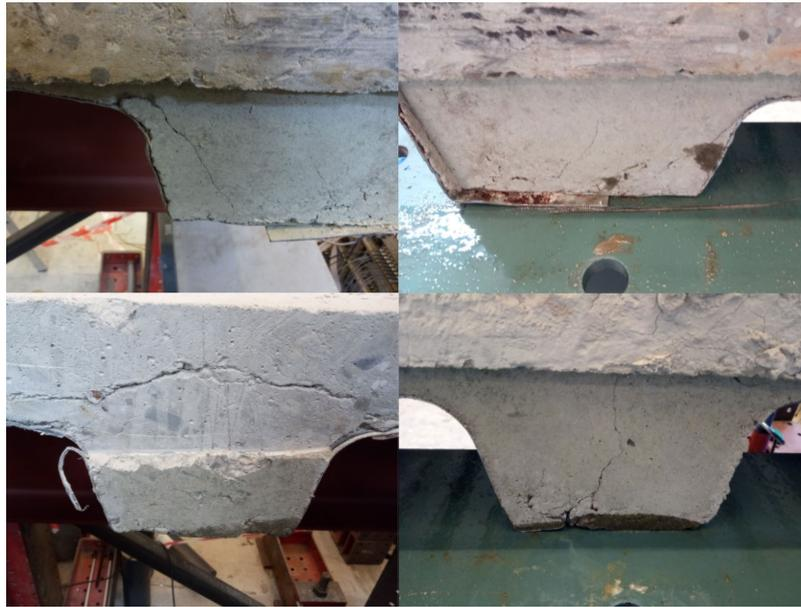
Figure 4.16: View on the cracks in the ribs along the longitudinal cut
