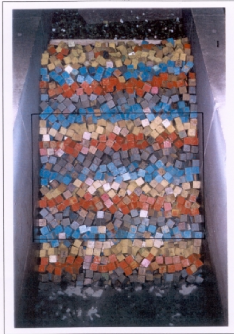
NDC - dumped, area of picture 2 used for determining roughness
