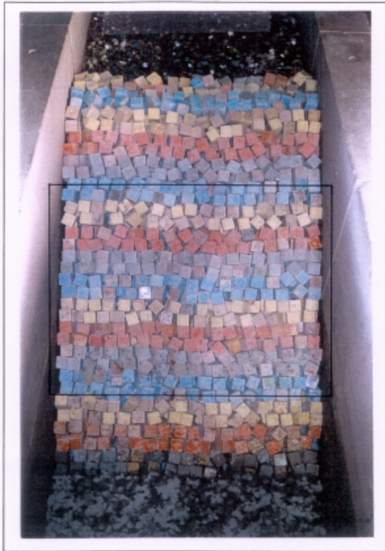
NDC – placed, area of picture 1 used for determining roughness
