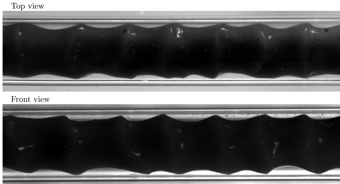
Figure 7.1: Typical core-annular flow pattern for Q_o = 0.35 l/s, C_w = 20\% and \nu_o \approx 2510 cSt ( T_o \approx 23.4^\circ\text{C} ).
