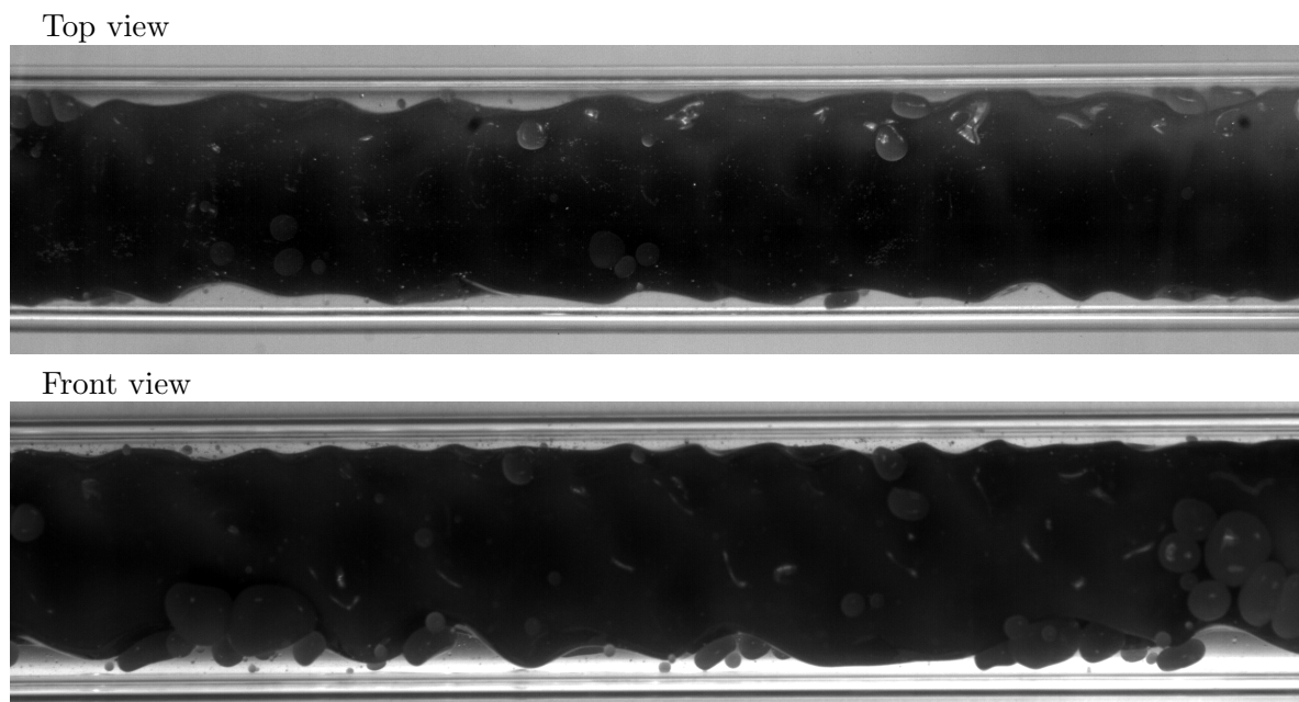
Figure 7.4: Typical core-annular flow pattern for Q_o = 0.35 l/s, C_w = 20\% and \nu_o \approx 440 cSt ( T_o \approx 47.6^\circ\text{C} ).
