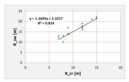
Figure E.15: Relation between the crane footprint radius and swing radius.
