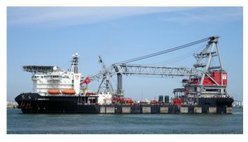
Figure A.2: The Oleg Strashnov vessel, fitted with a single 5000 mton capacity crane.
