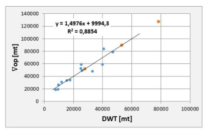
Figure E.3: Monohull: relation between the operational displacement  $(\nabla_{op})$  and deadweight tonnage (DWT).
