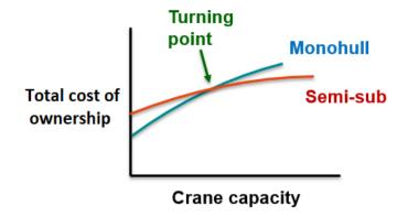
Figure 2.3: Schematic impression of the cost (Operational and capital) that depends on the crane capacity of the vessel.
