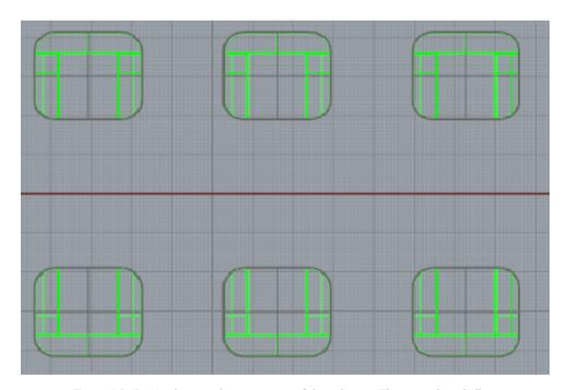
Figure 4.6: Semi-sub general arrangement of the columns. There are three ballast tanks fitted per columns. The rest of the space is reserved for other items such as thruster rooms and chain lockers.
