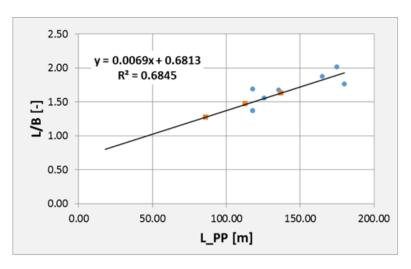
Figure E.10: Semi-submersible: Length-width ratio as function of the vessel length.
