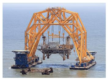
Figure A.6: A multihull heavy lift vessel, consisting of two hulls connected by a crane structure in between.
