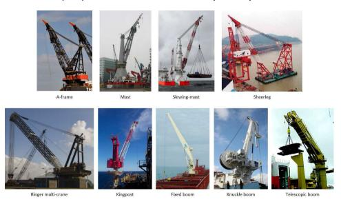
Figure F.1: The different types of cranes that can be used on-board ships. [17]
