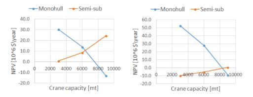
Figure 10.3: NPV calculations for the North Sea(left) and West Africa(right) environment for both vessel types.
