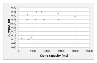
Figure E.9: Semi-submersible: Waterplane area ratio as function of the crane capacity.
