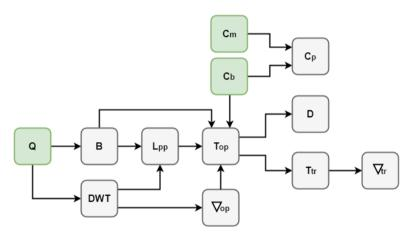
Figure 3.1: Main parameters selection flow for the monohull designs. Green boxes mean it is either an input or chosen parameter.
