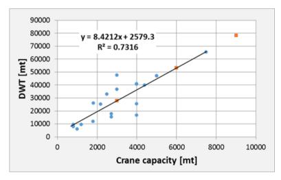
Figure E.2: Monohull: relation between the crane capacity (Q) and Deadweight tonnage (DWT) of the vessel.
