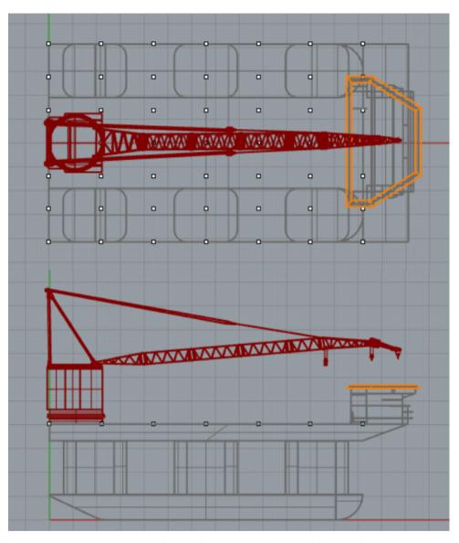
Figure 4.4: Semi-sub general arrangement drawings of the main deck.
