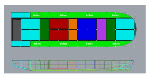
Figure 3.6: Monohull general arrangement of the internal components, including the ballast tanks.
