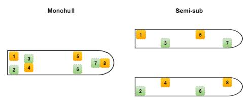
Figure 8.2: Monohull (left) and Semi-submersible (right) thruster division over the switchboards.
