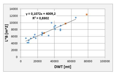
Figure E.4: Monohull: relation between the length times width  $(L_{PP} \cdot B)$  and deadweight tonnage (DWT).
