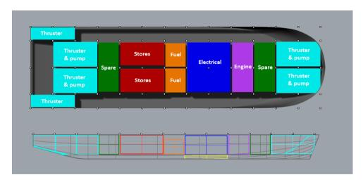
Figure 3.5: Monohull general arrangement of the internal components, except the ballast tanks. All items are separately indicated. The fresh water tanks can be seen in the bottom picture below the other items.
