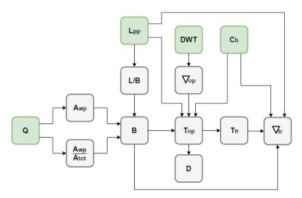
Figure 4.1: Main parameters selection flow for the semi-sub designs. Green boxes mean it is either an input or chosen parameter.
