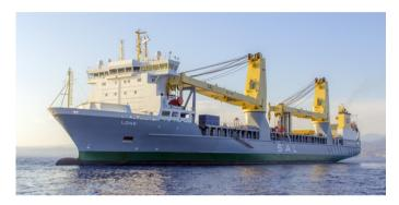
Figure A.1: The SAL type 176 vessel, fitted with 2 cranes of 700 mton capacity.
