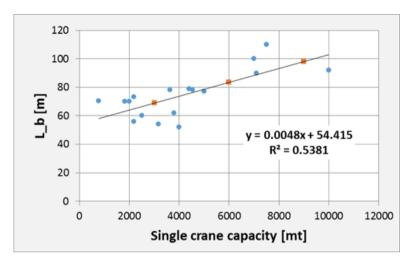
Figure E.16: Relation between the main boom length and single crane capacity.
