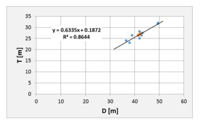
Figure E.12: Semi-submersible: relation between the operational draft  $(T_{op})$  and depth (D).
