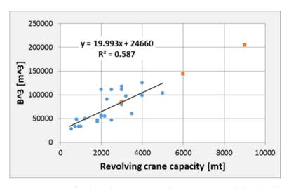
Figure E.1: Monohull: relation between the revolving crane capacity (P) and width  $(B^3)$  of the vessel.
