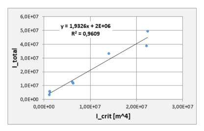
Figure E.7: Semi-submersible: Relation between the critical area moment of inertia  $(I_{crit})$  and total area moment of inertia  $(I_{total})$ .
