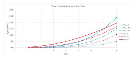
Figure 8.8: Required DP power for a range of environmental conditions for both vessel types, for a few headings.
