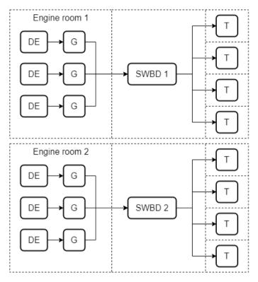
Figure 8.1: Sketch of the propulsion system layout. DE=Diesel Engine, G=Generator, SWBD=Switchboard, T=Thruster
