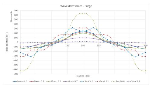
Figure 8.5: Wave drift surge forces for both vessel types for a selection of wave periods.
