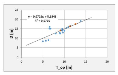
Figure E.5: Monohull: relation between the operational draft  $(T_{op})$  and depth (D).
