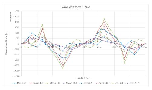
Figure 8.7: Wave drift yaw forces for both vessel types for a selection of wave periods.
