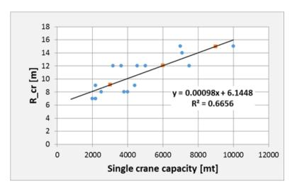
Figure E.14: Relation between the single crane capacity and footprint radius.
