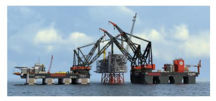
Figure A.7: Two multihull semi-submersible ships carrying out an operation.
