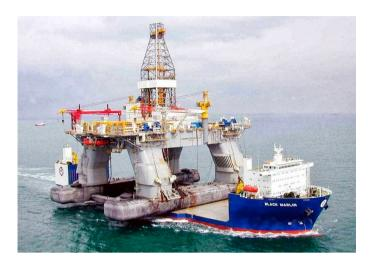
Figure A.5: The Black marlin, a monohull semi-submersible ship, capable of lifting cargo that floats over its deck.
