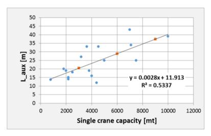
Figure E.17: Relation between the auxiliary+whip boom length and single crane capacity.
