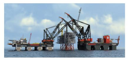
Figure 1.2: Two multihull semi-submersible ships carrying out an operation. On the left the Thialf with a combined crane capacity of 14200 tonnes, and on the right the Sleipnir, which is still under construction, with a combined crane capacity of 20000 tonnes
