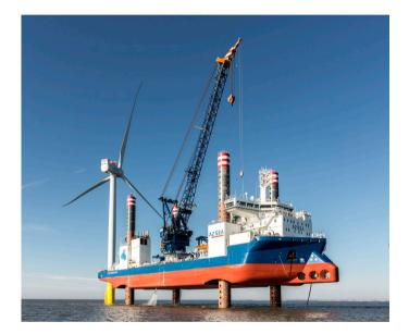
Figure A.4: A jack-up vessel, capable of lifting itself above the water surface.
