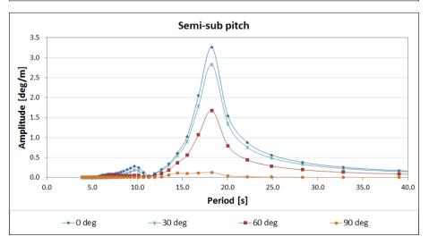
Figure 7.2: Semi-sub RAOs for heave, pitch and roll in the North-sea.
