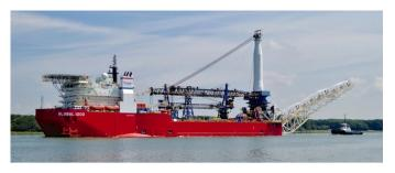
Figure A.3: The Global 1200 vessel, capable of heavy lift and pipelay operations. The crane has a 1200 mton capacity.
