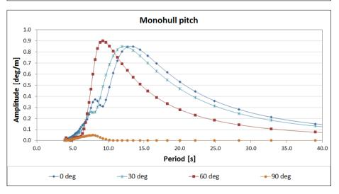
Figure 7.1: Monohull RAOs for heave, pitch and roll in the North-sea.
