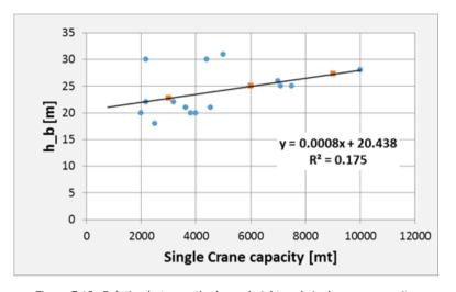
Figure E.18: Relation between the boom height and single crane capacity.
