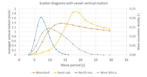
Figure 7.3: The north-sea and West africa wave scatter plot (blue and grey lines), together with an averaged vertical motion plot for both 6000 mt vessels.
