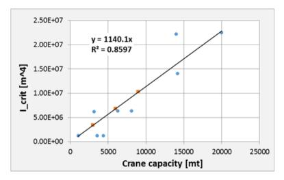
Figure E.6: Semi-submersible: Relation between the critical area moment of inertia  $(I_{Crit})$  and total crane capacity (Q).
