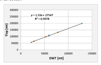
Figure E.11: Semi-submersible: Operational displacement as function of the DWT.
