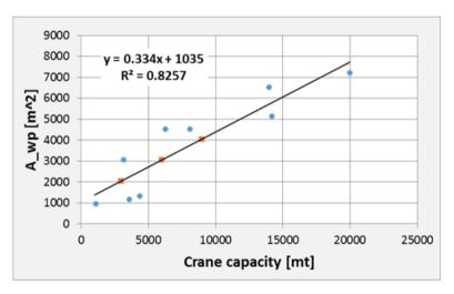
Figure E.8: Semi-submersible: Waterplane area as function of the crane capacity.
