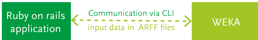
Figure 18: Communication between Ruby on Rails application and WEKA is performed via command line interface, data input for WEKA is formatted in .arff file format.
