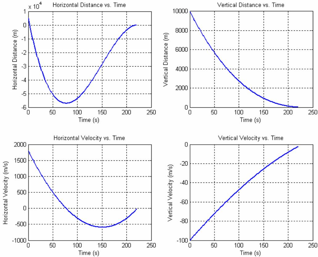
**Figure 8. Variations of State Variables ( $x_0=5000\text{m}$ ,  $v_0=1800\text{m/s}$ ).**
