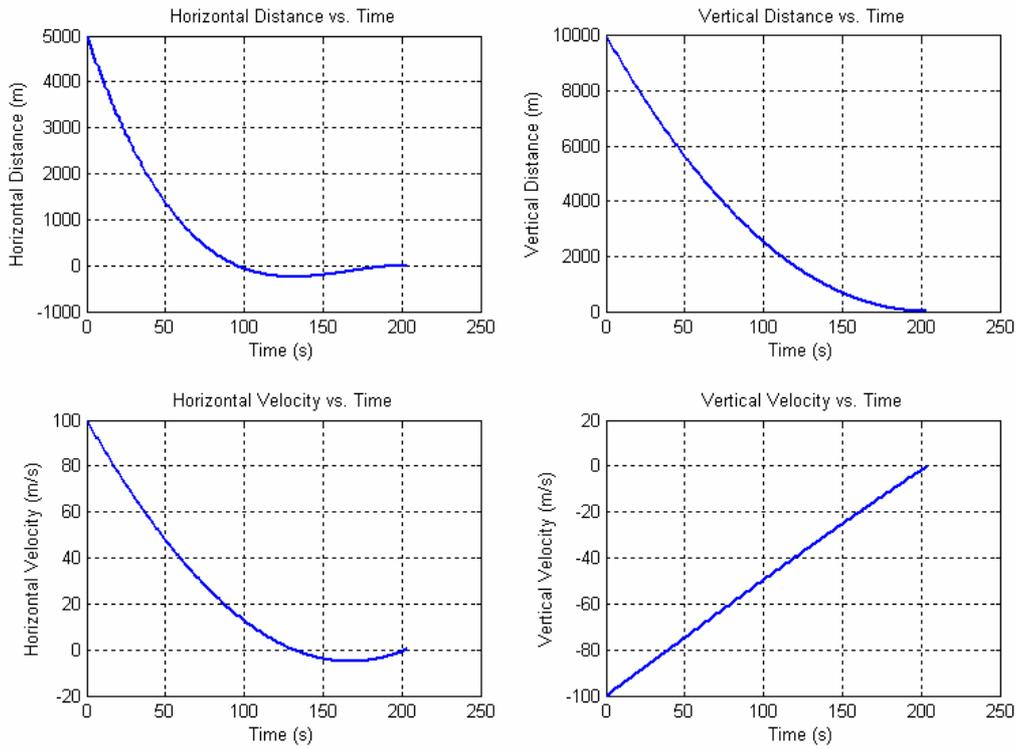
**Figure 9. Variations of State Variables ( $x_0=5000\text{m}$ ,  $v_0=100\text{m/s}$ ).**
