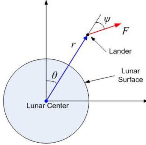
Figure 4. State Variables for Equations of Landing.
